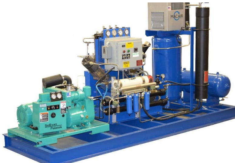
NITROGEN GENERATOR PACKAGE COMPLETE WITH FEED-AIR COMPRESSOR, AIR DRYER AND 3600 PSIG BOOSTER COMPRESSOR FOR CYLINDER FUELING
